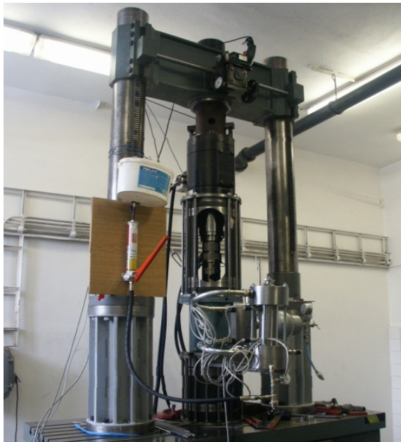
Fig. 6. Final system: load frame with two linear hydraulic units, delimitation cages, model of hydraulic unit and damper chamber
